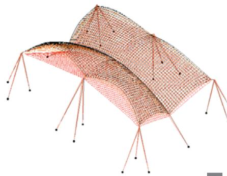
Figure 5. Deflection under longitudinal upward wind loading
